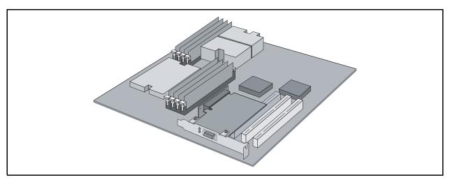
Figure 4-6. Assembled PCIe HCA with Riser
